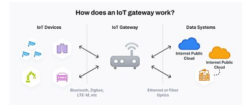
Fig. 1. IoT devices connect with cloud services with edge and gateways.
