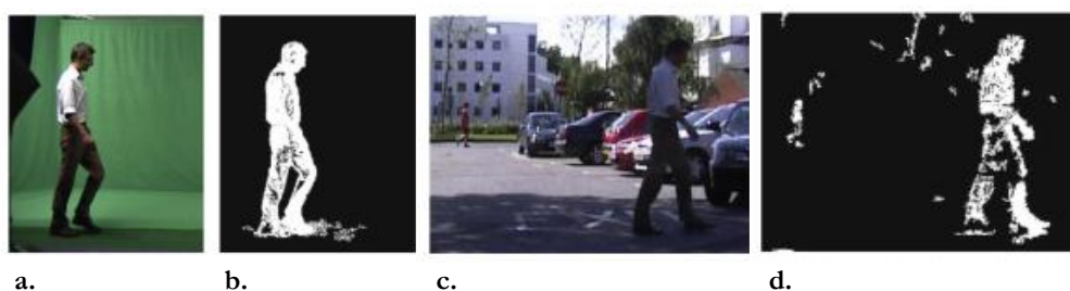
Fig. 2. Feature extraction for object detection; a. indoor data, b. extraction from indoor data, c. outdoor data, d. extraction from outdoor data.
